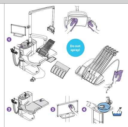
\*Before cleaning the instrument console, lock the touch screen.
