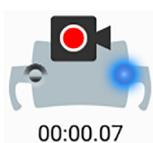
**Planmeca dental unit:** When recording is going on, the camera indicator light on the **Solanna Vision** button in the main window blinks to indicate that recording is going on.
