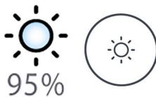
**Control panel:** Press and hold the **Operating light** button to adjust the operating light intensity.
