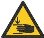
Warning, crushing hazard: hand (Standard ISO 7010).
