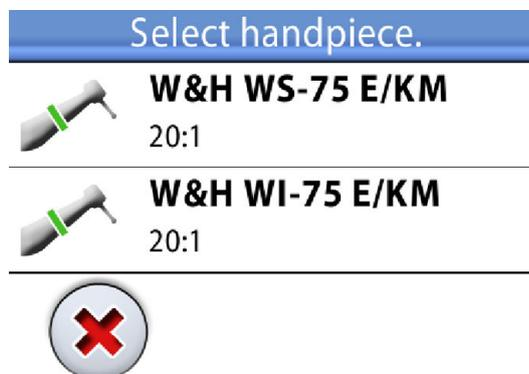
Press on the correct handpiece to select it. The window closes and the instrument settings and the handpiece information on the control panel change accordingly. To close the window without selecting a handpiece, press **Close**.
