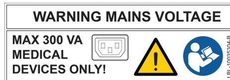
The multiple socket outlet (MSO) is reserved for medical devices that comply with the IEC 60601-1 standard. The MSO is available as an option.
